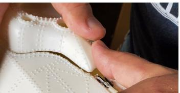
Once the upper edge is fully cured and solidly installed, place the lower hull against the lower edge of the salon bubble and use the same process of placing mounting tabs and then methodically tacking the edge of the bubble against the lower hull. Once perfectly in place, commit with a full bead of thick CA.
