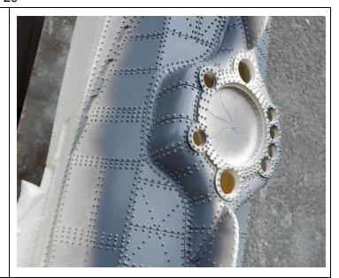
Check the spacing of the upper and lower hull sections by using the side keels. Use the supplied plastic to create spacers of the correct width and then glue the upper and lower hulls together at these spacer points.
