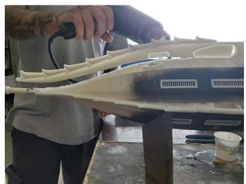
Properly done, there should be very little in the way of gaps to address with the side keels. Use thick CA along the seam and wipe clean to glue the parts together and fill any small gaps.
