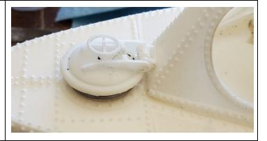
In the same manner, the lower ventral dive hatch is set in place, the mounting bracket is set in place, and the bracket secured to the lower hull permanently.
