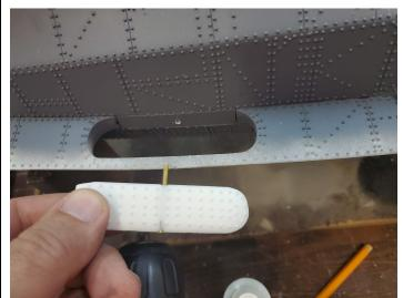
Properly done, your dive plane should have a minimum of 30 degrees of travel up and down. A drop of thick CA on the outside exposed rod will hold it in place.
