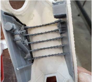
7 Once you are satisfied with the placement of the interior detail pieces, install the ship's wheel and dive levers.
