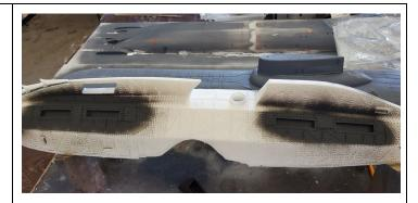
19 Insert the ballast grates into the recesses, ensuring you fully press them flush with the hull prior to securing with thin CA glue
