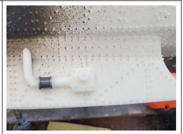
The phospohoric atomizer part is installed in a similar manner on the rear lower keel
