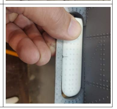
Drill a 1/16" hole through the center of the diveplane. I find that you will want to file a flat spot on the edge of the part prior to trying to start your pilot hole in order to stop bit wander.
