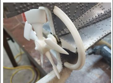
Mark out the propeller guard at 45 degree increments from vertical and horizontal. You can use a compass or calipers to measure the center of each upper and lower half of the left and right guards.
