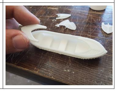
The two smaller sections are stacked together and glued. If you use a flat surface, you can assemble this by stacking the parts and glueing together with thin CA
