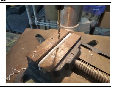
Mark out the placement of the 1/16": hole for the side keel and hull, ensuring that it is aligned to your previous marking and centered on the width of the side keel.
