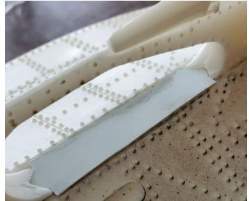
If you are making your dive planes practical, place them in the open holes in the side keel and ensure you have a proper perimeter gap by sanding/filing the edges.
