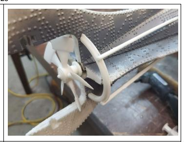
The rudder is installed into the recesses in the upper and lower tail. Ensure smooth swiveling of the propeller. You may need to place some small washers on the upper and lower shafts in order to get perfectly centered placement between the upper and lower tail pieces.
