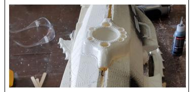
Done properly, you will have a very minimal gap, and the thick CA works well as a gap-filler. Use primer on the finished seam to check for gaps, bubbles or voids
