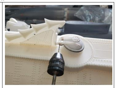
The forward lower keel mechanism gets installed by drilling out the orientation holes in the lower hull and aligning the parts to them. The piping extends from this part toward the bow.
