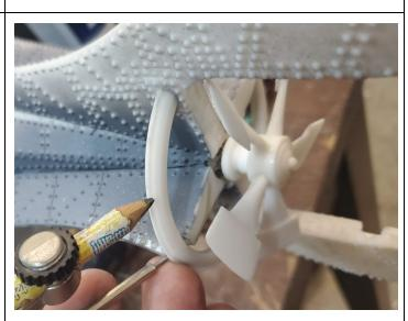
The propeller guard struts are installed at the marked points using thick CA. The bases are adhered to the pads located on the upper and lower hulls.
