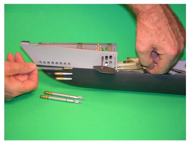
**Charging the Weapon** The system is so designed that you can not charge the weapon off-launcher. If the launcher is wet from recent immersion, insure that you blow out the little bit of water trapped within the face of the launcher charge fitting – failure to do so will result in water being driven into the system plumbing during the charging operation. If any water gets within the weapon it may flash to ice crystals as the propellant
