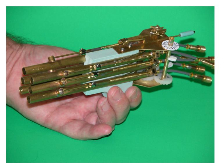
But, what if you wish to employ the Caswell-Merriman mechanical launchers in, say, a six-tube nest like what I've done for my GATO? In that case: you get creative! To help you out, I'll give you a little insight on how I designed, built, and installed a launcher trigger tripping mechanism onto the bow launcher nest of my 1/72 Revell GATO model submarine.
