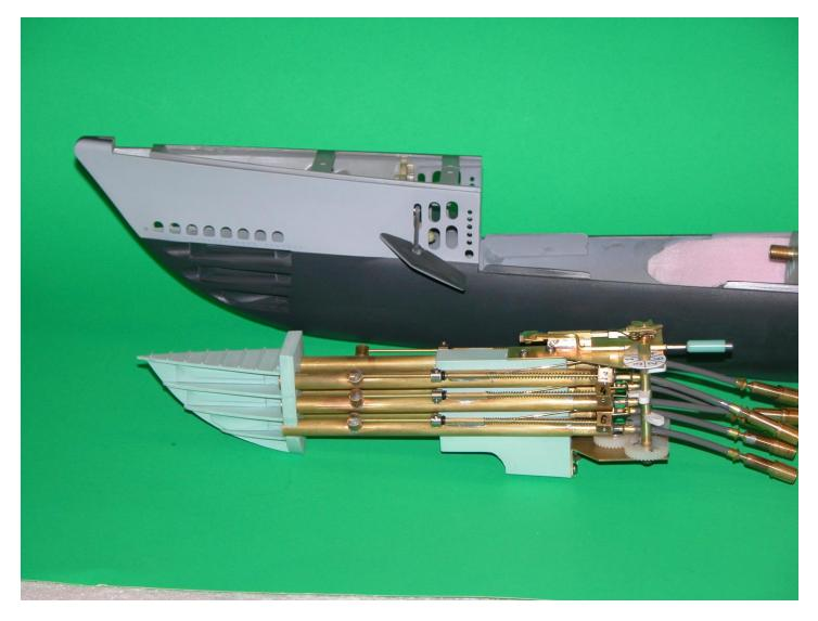
As you can see, things are a bit tight in the bow of the GATO with a complete set of launchers and the attached launcher trigger tripping mechanism.
