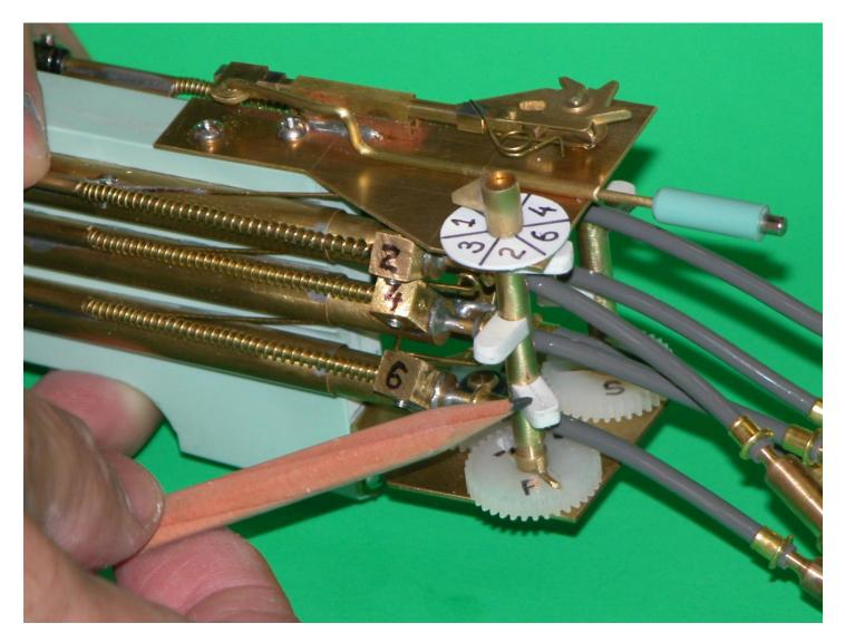
Anyway ... that's how I came up with a single-servo launcher trigger tripping mechanism. Hope it gave you some good ideas. Have a bottle of heavy-duty aspirin nearby when you start in on this gadget!
