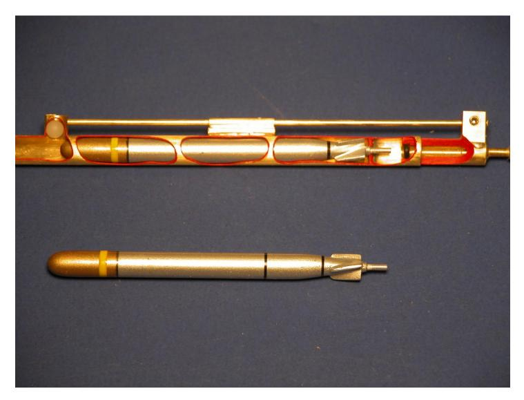
The launcher is designed for easy disassembly should the need arise for adjustment or repair. We have provided spare O-rings, stop-bolt ball, and an extra wheel-collar set-screw. Note in the picture below an assembled launcher in the battery condition. A disassembled launcher is presented above the assembled launcher. This shot should pretty much tell you all you need to know about launcher design and operation.
