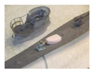
The same type horizontal snorkel head-valve is employed aboard the Revell 1/72 Type-7 kit with suitably sized float -- all fitting nicely under the magnetically attached fairwater. Note the flexible hose under the deck. The end of this piece of induction hose makes up to the Sub-driver mounted five-point manifold prior to securing the deck atop the models hull.
