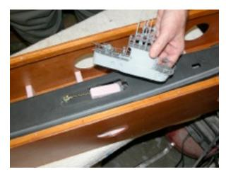
And here's the horizontal type snorkel head-valve installed aboard the beautiful Revell 1/72 GATO kit. The fairwater is secured atop the hull with magnets, permitting quick and easy access to the float and its flexible hose. Such access is needed to make/break the hose connection between the snorkel head-valve and the Sub-driver's five-point manifold under the float, glued atop the Sub-driver.
