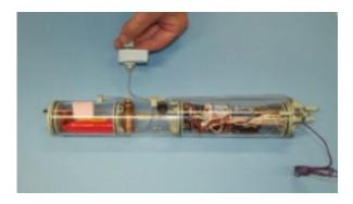
A short but long-of-cord float works to block off the head-valve when water reaches the sail of the Trumpeter 1/144 SEAWOLF this SAS equipped Sub-driver is designed for.
