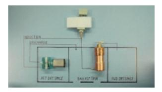
In this arrangement the Sub-driver's interior is an alternative source of air used by the LPB pump to empty the ballast tank.
