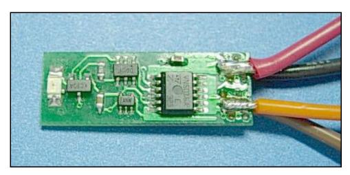
The last step in the soldering task is to clean all the solder joints with alcohol to remove any solder flux residue. Use a stiff brush and plenty of alcohol. (A clean acid brush with bristles trimmed to 1/4" works really well for this.) Finally, cover up the MMS-10 with the provided heatshrink and apply gentle heat.
