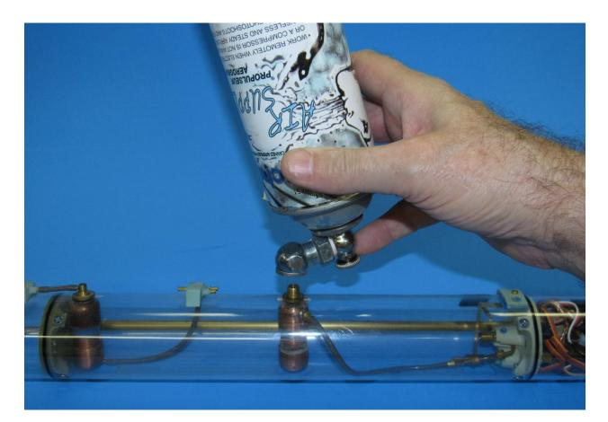
**MISSION** At The boating site tighten the bottle charge fitting valve and charge the bottle at the lake/pool shortly before placing the model in the water.
