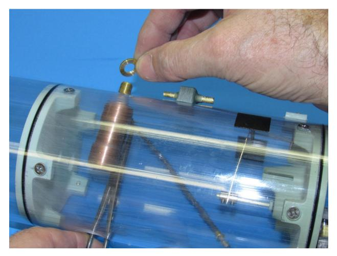
Screw down the securing nut a few threads to keep the bottle from falling down into the ballast tank. Remove the hemostat and push on the bottom of the bottle with a finger as you hand tighten the securing nut. Don't use any tool to wrench down on the nut or you'll unseat the sealing o-ring. Hand-tight only!
