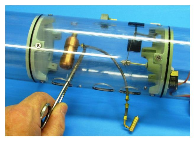
Remove the propel bottle securing nut and set it aside. Insure that the sealing oring remains atop the bottle.
