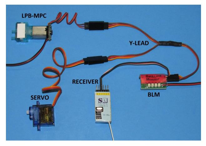
The above bread-board device layout represents a SAS type primary ballast subsystem. The only engagement the GBB has is through the linkage operated by the ballast servo, that linkage engaging the gas ballast device blow valve when the servo is over-positioned by the fail-safe device upon loss-of-signal. Normal transmitted commands do not over-position the servo, so no discharge of gas occurs during the 'blow' command.
