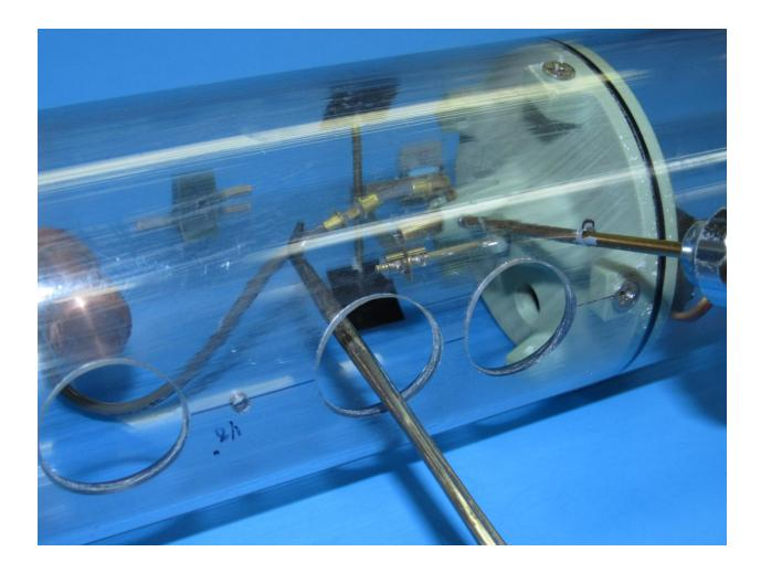
With the bottle now secured firmly to the top of the ballast tank, use the hemostat to grab and position the blow valve into the after ballast bulkhead blow-valve foundation. With the ballast sub-system servo in neutral, set the stem of the blow valve approximately 3/32" aft of the ballast linkage arm and secure the blow valve in place by **gently** tightening the 4-40 X 1/8" securing set-screw – the hex-wrench accessing that set-screw through a hole near the bottom of the ballast tank.
